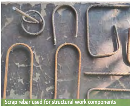
Scrap rebar used for structural work components
